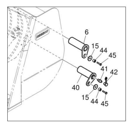
iii. Pin boss bolt, spacer, stopper - reference 45, 44, 15.
