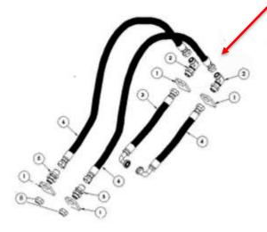
A *Jumper Hose Kit* is required to connect the piping kit directly to the attachment.
