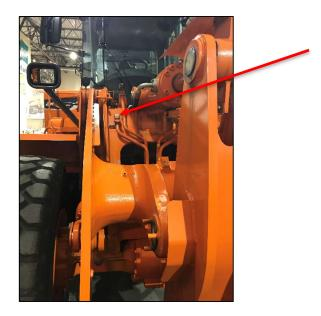
To connect and power the attachment, a *Piping Kit* is required on the lift arm.
